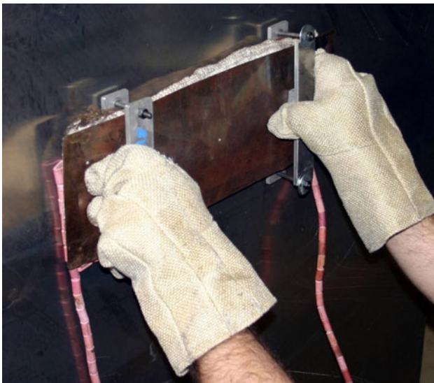
Fig. 7 Manual stabilization treatment of aluminum panel
